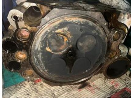
**Gambar**(pengecehan *exhaust valve*)
