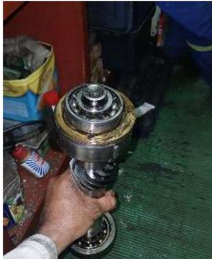
Gambar 8. Penggantian Bearing Vertical Shaft Fuel Oil Purifier
